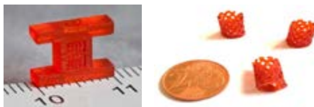
Figure 1: 3D printed test patterns out of a thiol/yne formulation; using Sudan II as a light absorber. (Scale on the left shown in cm).
