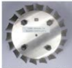
Figure 1. Hastelloy X manufactured blisks.
