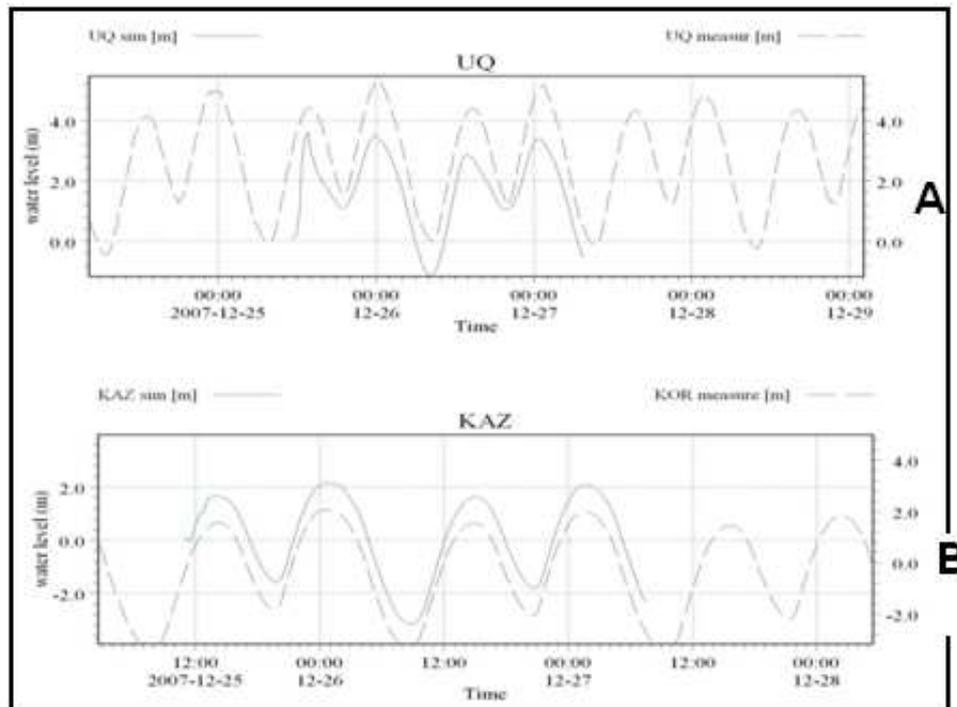
Figure 7. Comparison between water levels for simulation and measured. A- WL computed and measured in Umm Qasr site; B- WL computed and measured in Khor Al-Zubair site
