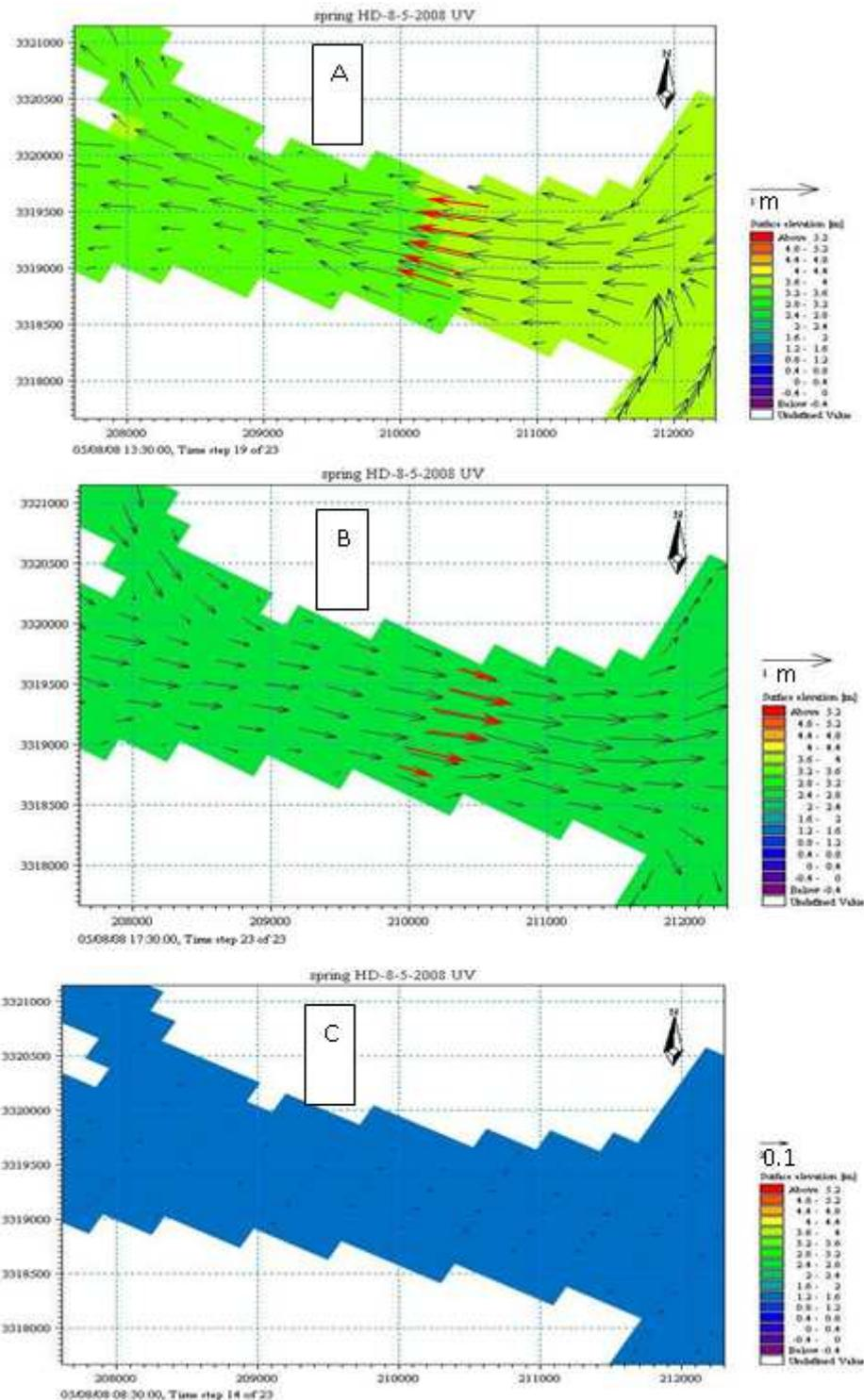
**Figure 8. Simulation (black arrow) and measurements (red arrow) of currents in Umm Qasr during the spring tide phase on 8-5-2008 A-flood B-ebb C-slack**
