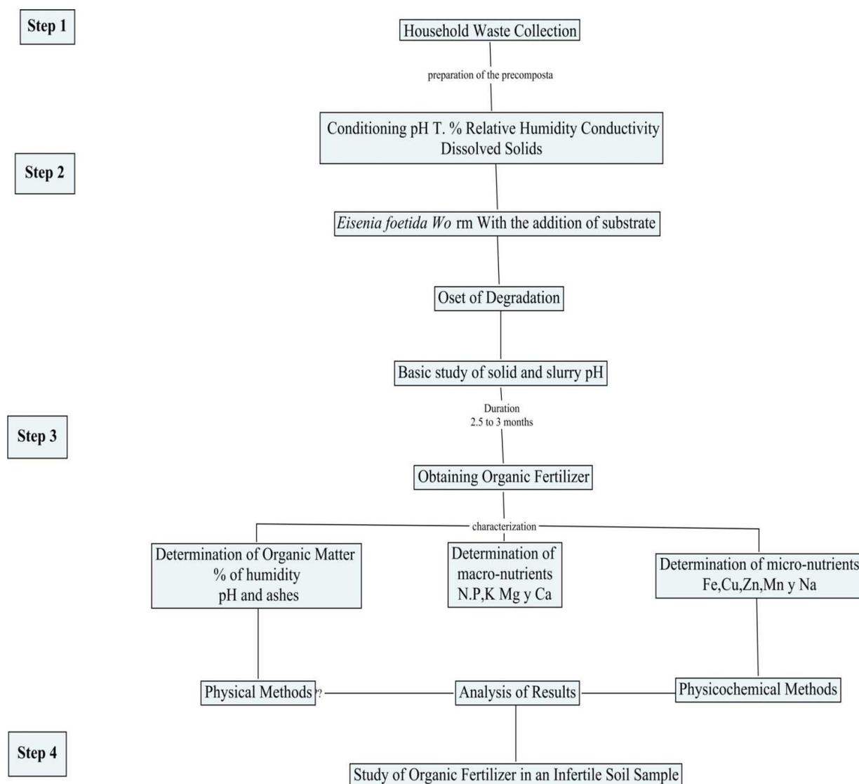
Fig.10 Experimental stages for obtaining compost from organic household waste
