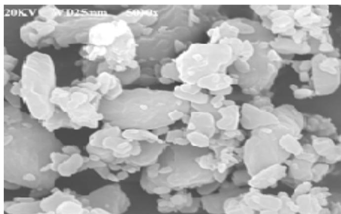
**Fig. 5 SEM of Ketoprofen bead**
