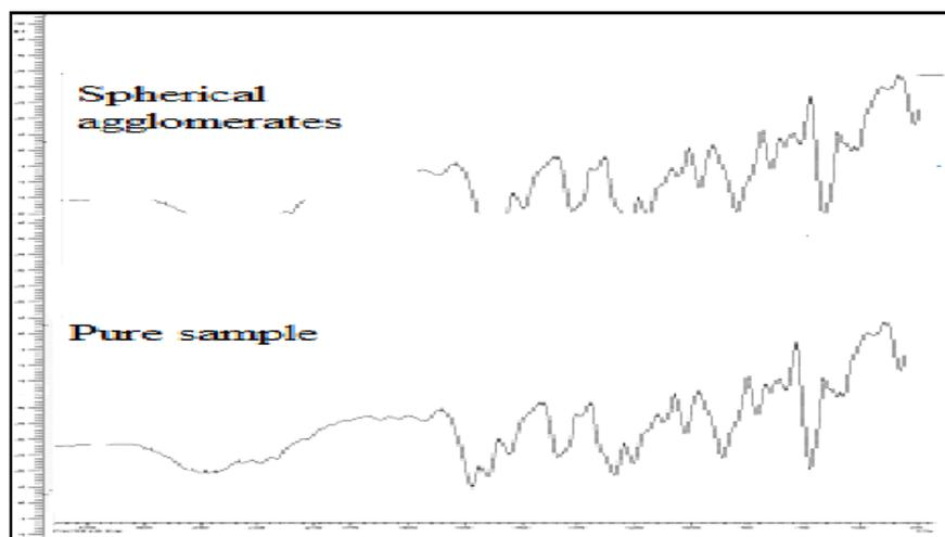
All the samples showed similar peak positions ( $2\theta$ ) in X-ray diffraction, formation of different polymorphs of ketoprofen was ruled out. However relative intensities of XRD peaks were modified (fig. 3). This could be attributed to the markedly different crystal habits of the samples (Table 4). Therefore the relative abundance of the planes exposed to the X-ray source would
