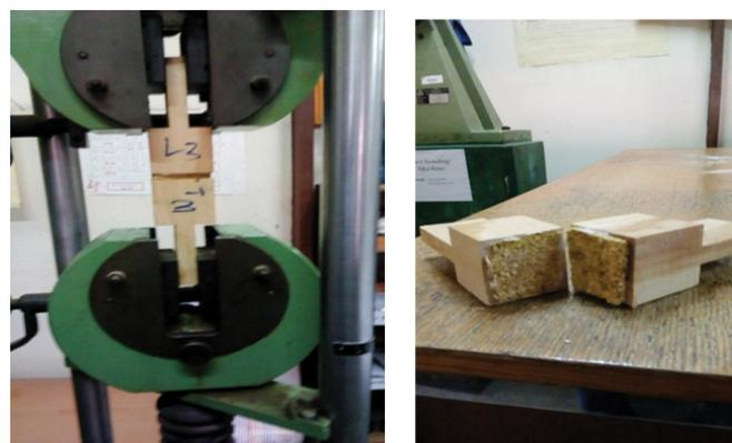
Figure 11 Test setup of IB test MC particle board.
