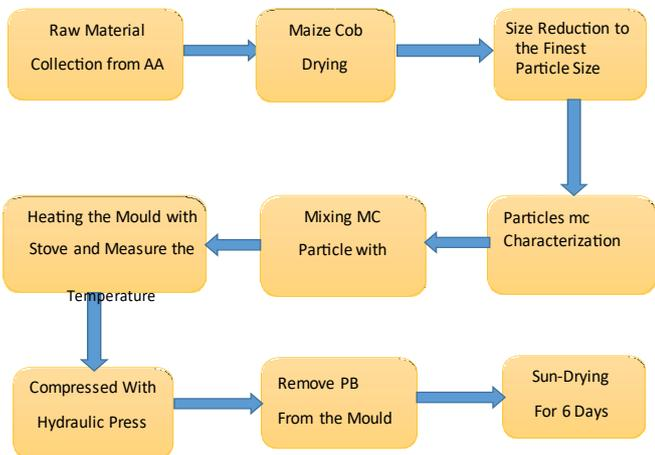
Figure 9 Experimental flow sheet diagrams of maize cob PB preparation.
