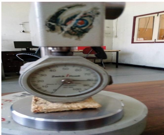
Figure 12 Hardness measuring setup of particle board.
