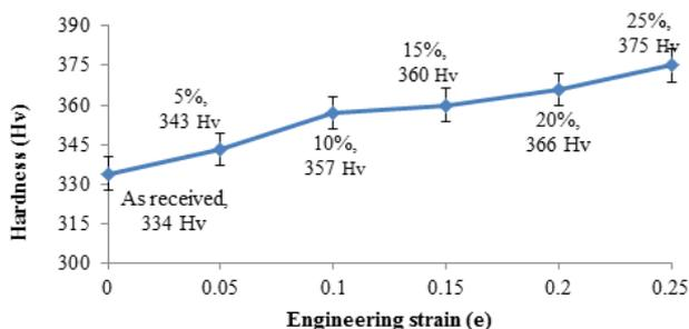
**Figure 4** Hardness of the as received and deformed samples of the Ti6Al4V with 0.01/s strain rate.
