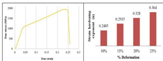
**Figure 1** Stress strain curves a) Engineering stress strain curves b) True stress strain curves c) strain hardening exponent ( $n$ ) of Ti6Al4V alloy.
