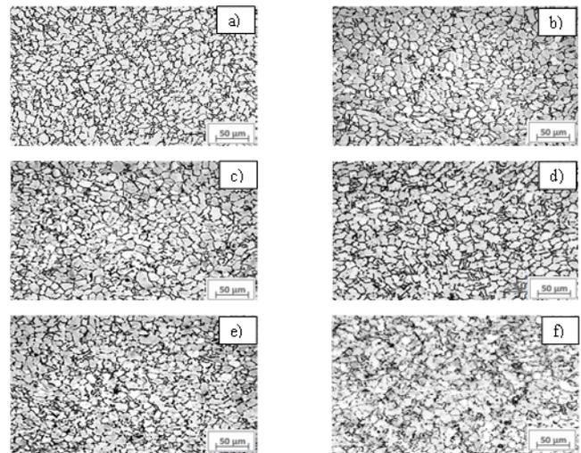
**Figure 5** Microstructures of the as received and deformed samples , a) As received sample b) 5% deformed c) 10% deformed d) 15% deformed e) 20% deformed f) 25% deformed.
