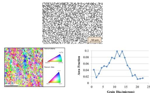
**Figure 2** a) optical micrograph b) EBSD IPF map c) Grain size of as received sample of Ti6Al4V alloy.
