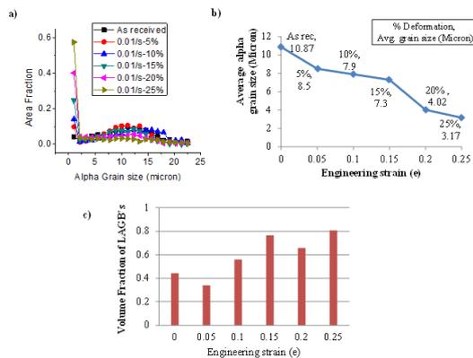
**Figure 3** a) Alpha grain size b) Avg. alpha grain size c) Volume Fraction of LAGB's (Low Angle Grain Boundaries) of the as received and deformed samples of the Ti6Al4V with 0.01/s strain rate.
