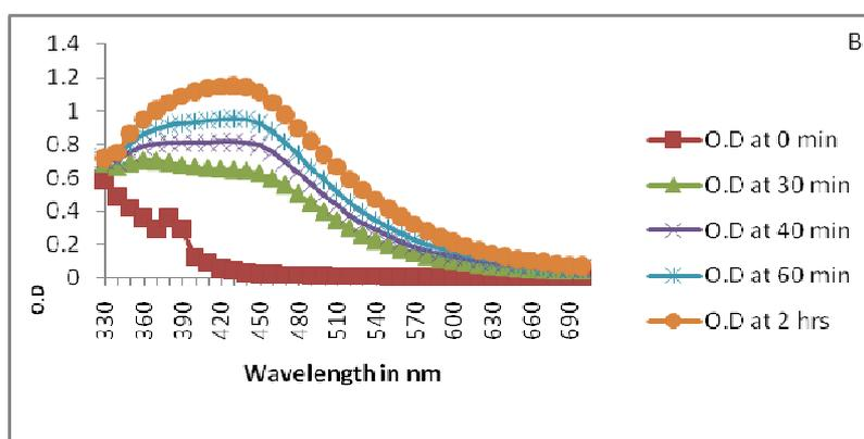
**Figure 2(B).** UV-visible spectrum of biosynthesized CR-AgNPs at different time interval, showed peak at 432 nm
