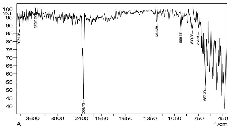
**Figure 3(A).** FTIR spectrum of biosynthesized CR AgNPs
