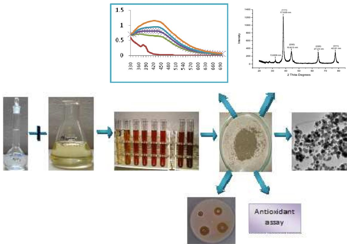
Green synthesis of silver nanoparticles using *C. roxburghii* stem extract and  $\text{AgNO}_3$ . Characterization by spectral analysis like UV-Vis, TEM, FTIR and XRD. Evaluation of antimicrobial and antioxidant potential
