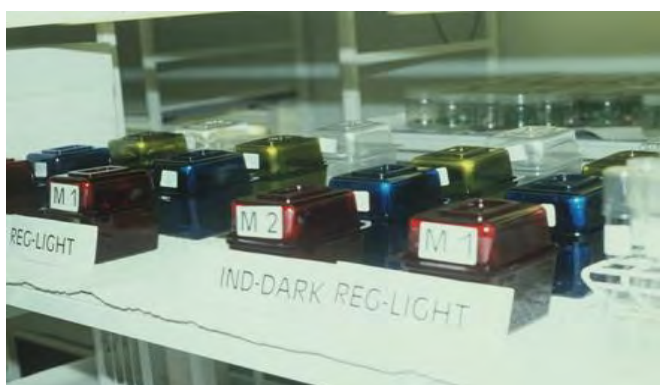
Figure 1 Layout and design of the tinted polystyrene containers.
