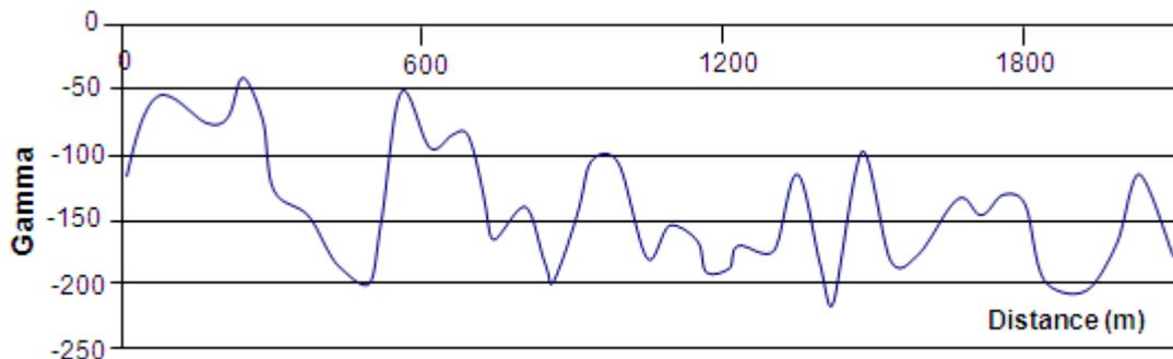
Figure 2d Total Relative Magnetic Intensity along Traverse 15 (NW - SE) of the study area
