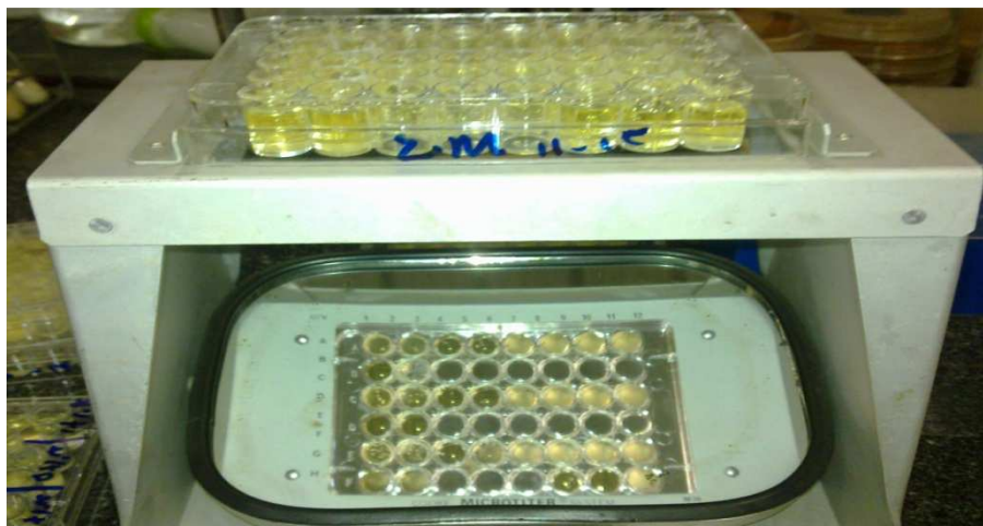
Figure 3: Use of a mirror to determine the MIC of C. albicans strains.
