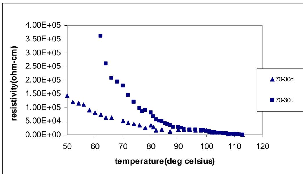
Figure 2: Resistivity Vs temperature of 70/30 doped (70-30d) and undoped (70-30u) films
