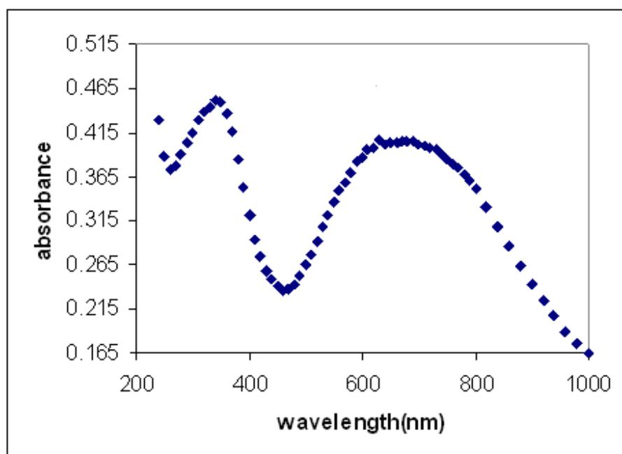
**Figure 1: Absorption band of 70/30 PVA/PAni blend**
