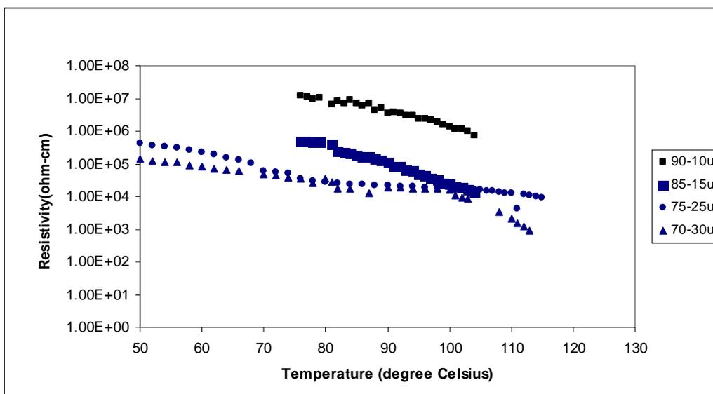
Figure 3: Variation of resistivity vs temperature of all undoped films of PVA/PAni blend
