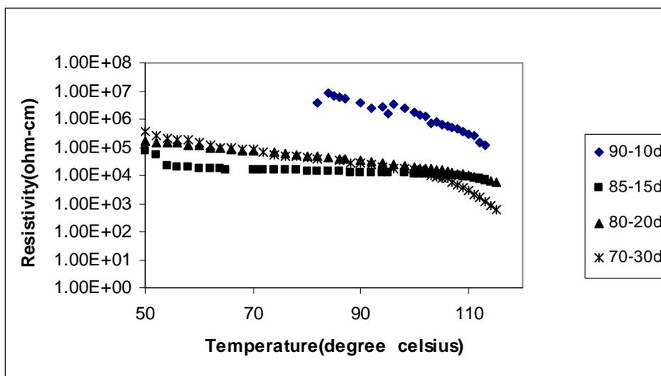
Figure 4: Variation of resistivity vs temperature of all doped films of PVA/PAni blend.
