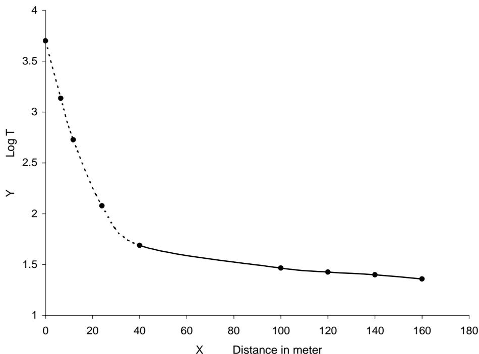
Fig 3 Temperature vs distance curve in Dikom fire
