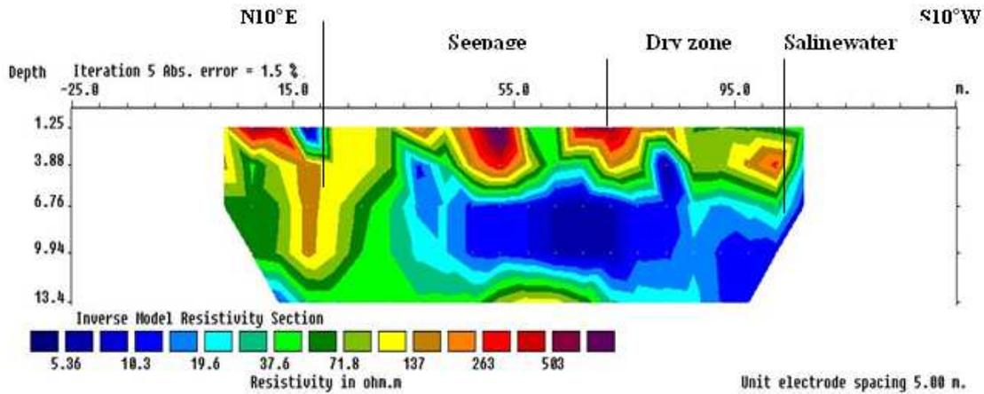
Fig. 3 2D electrical resistivity imaging pseudosection along profile 2 depicts the seepage zone around the embankment of freshwater storage reservoir.
