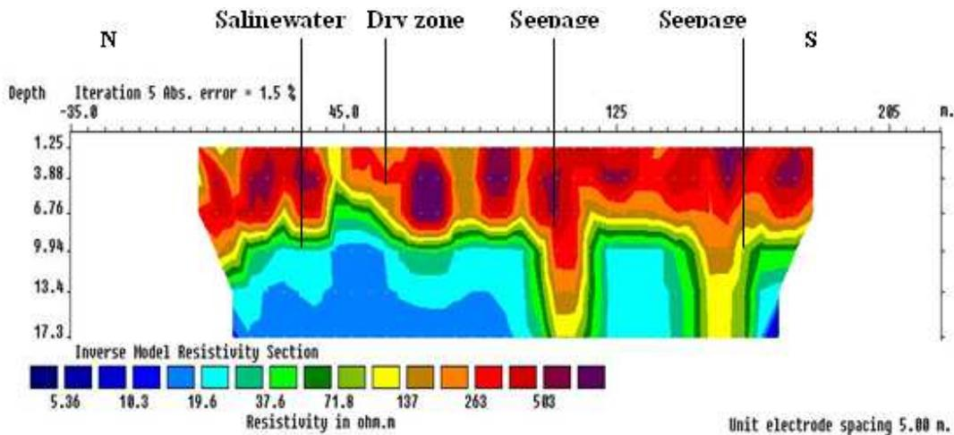
Fig. 4 2D electrical resistivity imaging pseudosection along profile 3 depicts the seepage zone around the embankment of freshwater storage reservoir.
