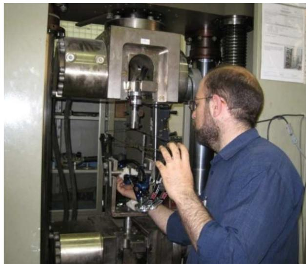
Fig 2. Tensile test of bows in Zwickmachine
