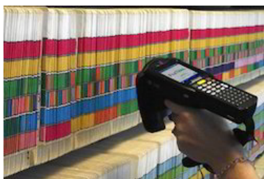
Figure 9: RFID scanner for detecting the patient medical record files.
