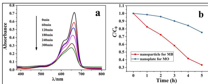
**Figure 8:** (a) Absorption spectra of MB photocatalytically degraded by AgInS<sub>2</sub> nanoparticle; (b) The relation between MB concentration and time photocatalytically degraded by AgInS<sub>2</sub> nanoparticle (the red curve), and the relation between MO concentration and time photocatalytically degraded by AgInS<sub>2</sub> nanoplate (the blue curve).
