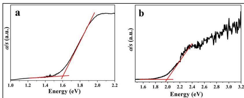
**Figure 7:** UV-vis diffuse reflectance spectrum of as-prepared products: (a) AgInS<sub>2</sub> nanoplate, synthesized at 120°C for 20 h using pyridine as the solvent, the bandgap is about 1.61 eV; (b) AgInS<sub>2</sub> nanoparticle, synthesized at 150°C for 17.5 h using 1-dodecanethiol as the solvent, the bandgap is about 1.98 eV.
