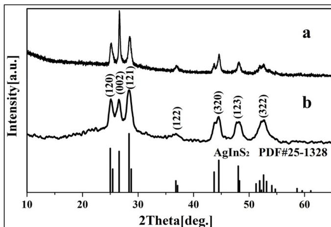
**Figure 1:** XRD pattern of as-prepared AgInS<sub>2</sub> samples: (a) 120°C/20 h, pyridine as the solvent; (b) 150°C/17.5 h, 1-dodecanethiol as the solvent.
