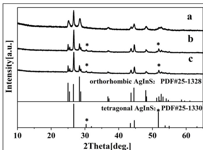
**Figure 4:** XRD patterns of products prepared at different temperature for 17.5 h using pyridine as the solvent: (a)  $150^\circ\text{C}$ , orthorhombic  $\text{AgInS}_2$ ; (b)  $170^\circ\text{C}$ , orthorhombic  $\text{AgInS}_2$  (major) + tetragonal  $\text{AgInS}_2$  (minor); (c)  $190^\circ\text{C}$ , orthorhombic  $\text{AgInS}_2$  (major) + tetragonal  $\text{AgInS}_2$  (minor)
