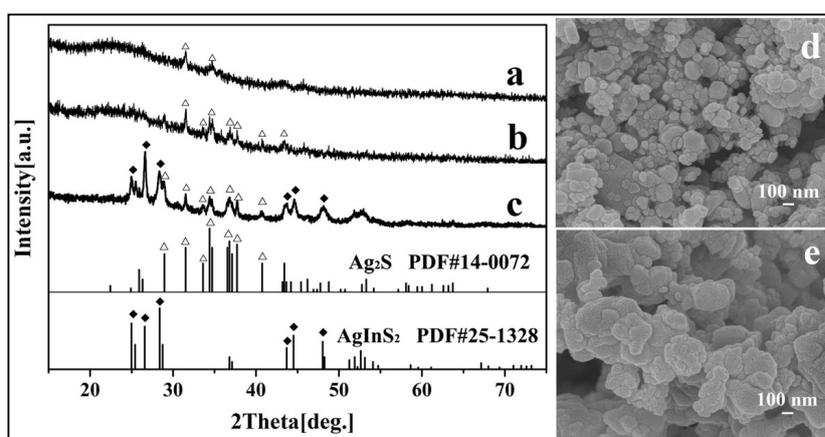
**Figure 3:** XRD patterns and SEM images of products prepared at 120°C for different time: (a) 5 h, weak diffraction peak, monoclinic Ag<sub>2</sub>S; (b,d) 10 h, monoclinic Ag<sub>2</sub>S, similar quantity of nanoplate and nanoparticle; (c,e) 15 h, the major orthorhombic AgInS<sub>2</sub> with minor monoclinic Ag<sub>2</sub>S, and the quantity of nanoplate is much larger than nanoparticle.
