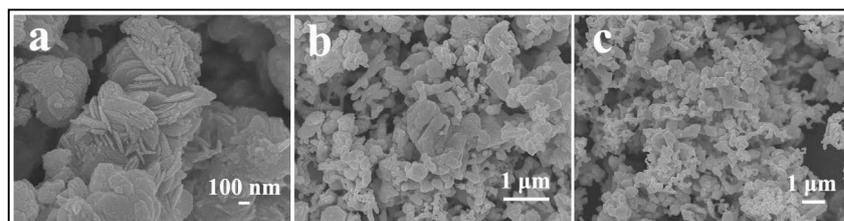
**Figure 5:** SEM images of products prepared at different temperature for 17.5 h using pyridine as the solvent: (a) 150°C; (b) 170°C; (c) 190°C.
