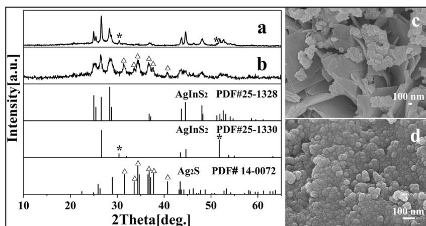
**Figure 6:** XRD patterns and SEM images of products prepared at 150°C for 17.5 h using other solvents: (a,c) ethylenediamine, orthorhombic AgInS<sub>2</sub> + tetragonal AgInS<sub>2</sub> (minor), square nanoplate + particle (minor); (b, d) oleic acid, orthorhombic AgInS<sub>2</sub> + monoclinic Ag<sub>2</sub>S, nanoparticle.
