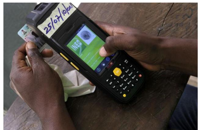
**Figure 4:** INEC Voters Identification System (IVAS) popularly called the Smart Card Reader (SCR)
