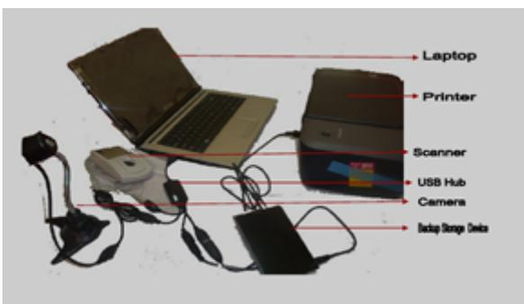
**Figure 3:** Direct Data Capture Machine currently being used for voters' registration
