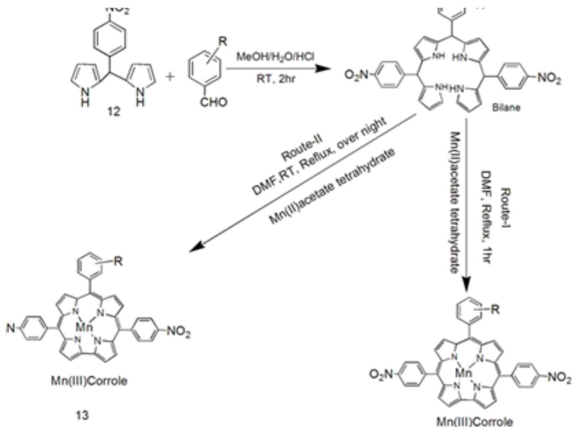
Figure 3: New synthetic methodology to yield manganese (III) corrole
