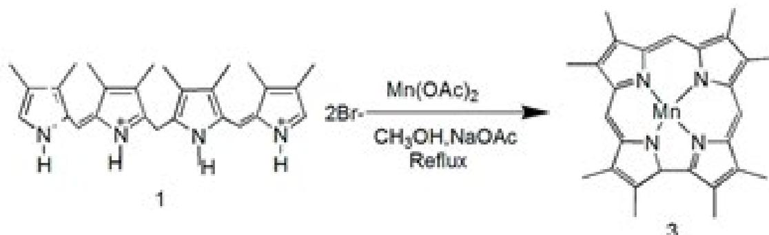
**Figure 1:** Cyclization of 1,19-dideoxybiladiene-ac with manganese (II) acetate tetrahydrate
