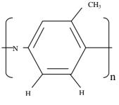
Fig.1 : structure of POT
