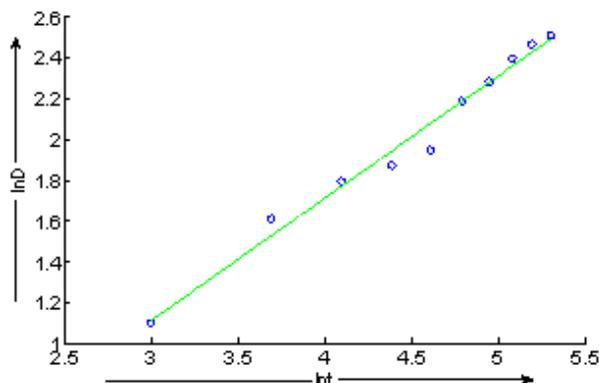
**Fig.13(a)** Plot of  $\ln D$  vs.  $\ln t$  for drug release of SMA-g-AAc hydrogel at 3.5pH
