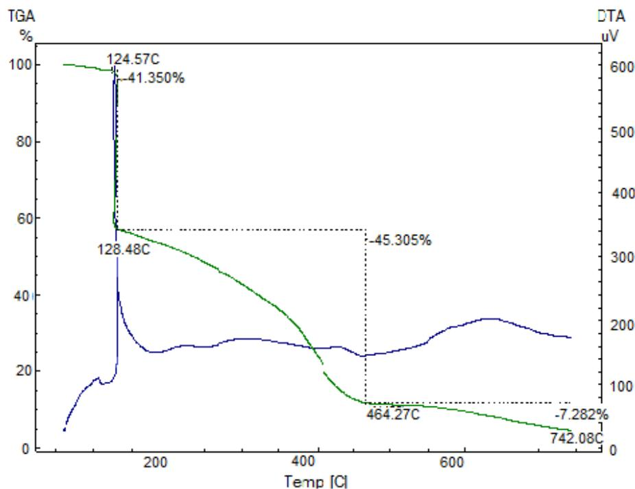
Fig.11(b). TGA of SMA-g- poly (AAc)
