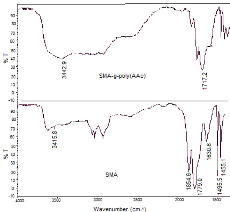
Fig.8. FTIR of SMA and SMA-g-poly(AAc)
