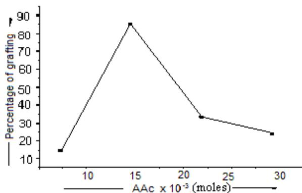
Fig.2. Effect of amount of AAc on percent grafting of AAc
