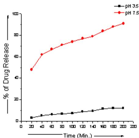
**Fig.12. Drug release from SMA-g-poly (AAc)**
