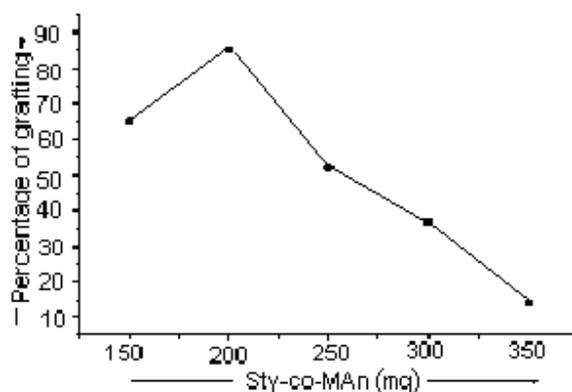
**Fig.1 Effect of amount of SMA on percent grafting of AAc**
