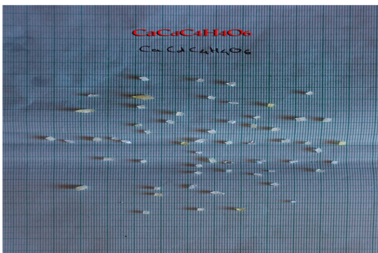
Figure 2 (a) Faint yellowish, Milky white, Transparent, Semitransparent, needle shape Well defined crystals of Calcium cadmium tartrate
