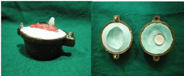
Figure 6: Investment of wax pattern followed by dewaxing.
