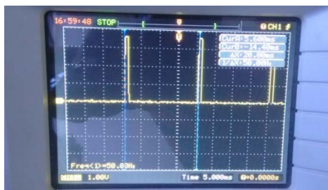
Fig 2(a): PWM signal with frame rate 50HZ
