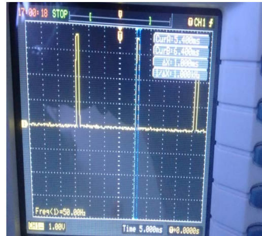
Fig 2(b): PWM signal with 1msec ON time
