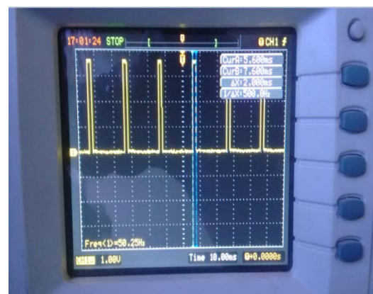
Fig 2(c): PWM signal with 2msec ON time
