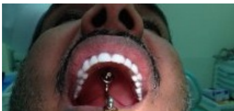
Figure 2 Hook in the geometric center of maxillary denture attached to strain gauge force meter.
