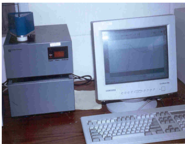
Fig 1. Diagram of Rapid visco analyser (RVA).
