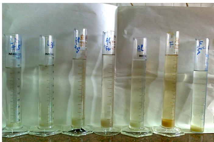
**Image (4) Picture of the effect of chemical coagulants optimum doses used and the aid of other techniques (Na- Ferrate oxidation and Ultra sound waves) on settling of micro algae *Microcyst,sp.***
