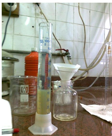
**Image (5) illustrating the degree of clear in supernatant when using pre-ultrasound treatment and Alum coagulation.**
