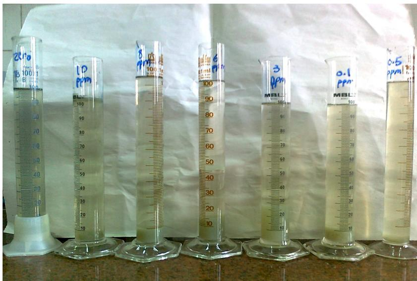
Image (2) illustrating the reduction of  $\text{FeCl}_3 \cdot 6\text{H}_2\text{O}$  dose and the clearly of the supernatant from the yellow color.
