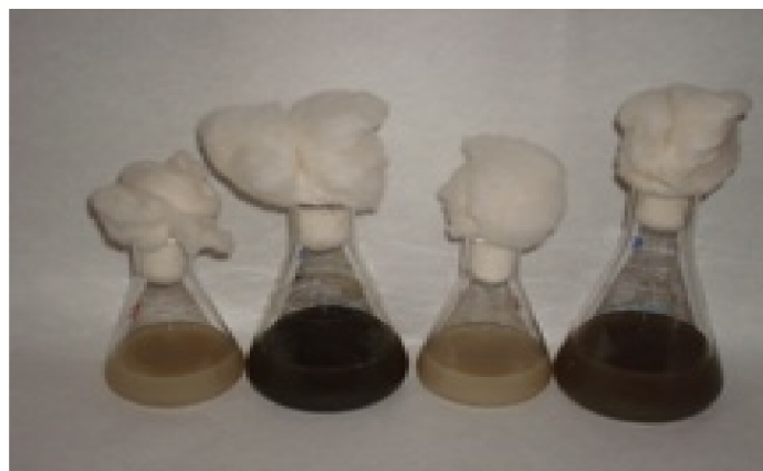
Figure 2. Appearance of brown color from off white indicates the formation of SNPs
