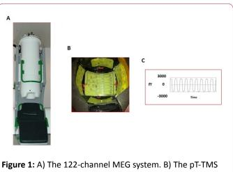
**Figure 1:** A) The 122-channel MEG system. B) The pT-TMS electronic device. C) The frequency output of the device using an oscilloscope (1 fT=10<sup>-15</sup> Tesla).
