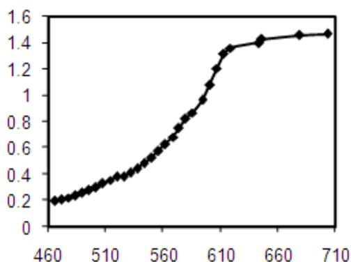
Fig. 9 Plot of  $f(\alpha)$  Vs. temp. for Zn-doped doped  $\text{PbI}_2$
