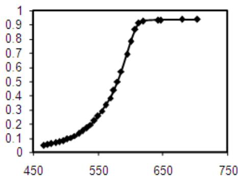
Fig. 5 Plot of  $\alpha$  Vs. temp. for Zn-doped  $\text{PbI}_2$
