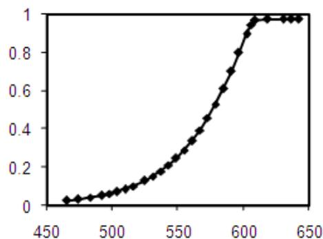
Fig. 4 Plot of  $\alpha$  Vs. temp.  $^{\circ}\text{C}$  for Al-doped  $\text{PbI}_2$
