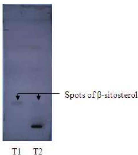
Figure 2: Photographed chromatoplate after derivatization with Liebermann-Burchard reagent.
