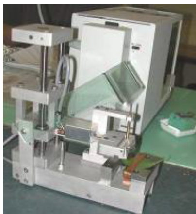
Figure 5: Leaf toughness tester.
