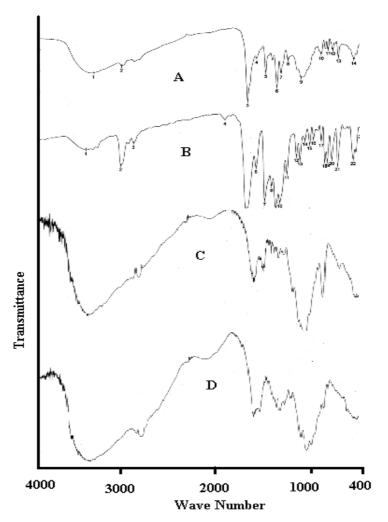
Figure 1: FT-IR spectra of A) Clobazam loaded chitosan microspheres B) Clobazam C) Blank microspheres D) Chitosan
