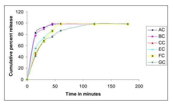
Figure 3: Cumulative percent release of clobazam in 0.1 N Hydrochloric acid (pH 1.2) from drug loaded microspheres
