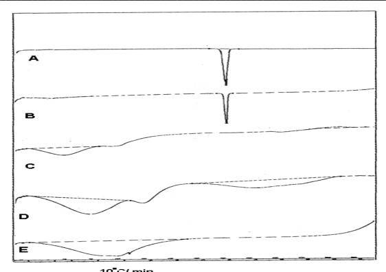
**10<sup>-</sup>**Cf min Figure 4: Differential scanning calorimetry (DSC) thermograms (A) clobazam (B) Physical mixture of clobazam and blank microspheres (C) clobazam loaded microspheres (D) blank microspheres (E) chitosan
