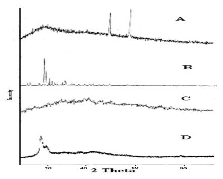
Figure 5: X-Ray Diffraction pattern of A) Clobazam loaded microspheres B) Clobazam C) Blank microspheres D) Chitosan
