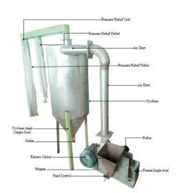
Figure 2: A milling system with pneumatic conveyor and cyclone
