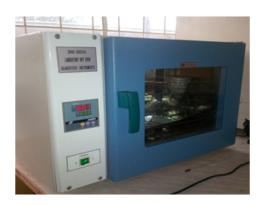
**Figure 4:** Laboratory oven (search tech instrument DHG-9053A)
