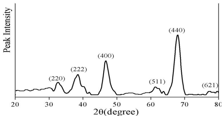
**Figure 2:** XRD pattern of a synthesized  $\gamma\text{-Al}_2\text{O}_3$  NPs.
