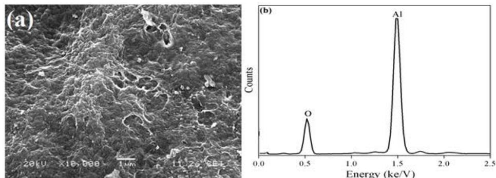
**Figure 3:** (a) SEM image of synthesized  $\gamma$ -Al<sub>2</sub>O<sub>3</sub> NPs (b) EDX spectrum of synthesized  $\gamma$ -Al<sub>2</sub>O<sub>3</sub> NPs.
