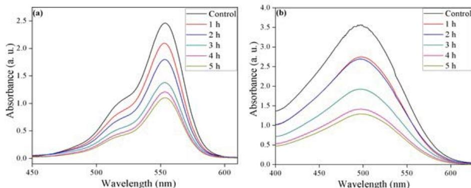
**Figure 4:** UV-vis absorption spectra of RhB (a) and CR (b) aqueous solution in the presence of  $\gamma$ -Al<sub>2</sub>O<sub>3</sub> NPs at different irradiation times.
