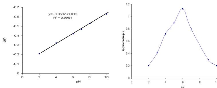
**Fig.-1: (A). The linear relation between  $E_p$  and pH; (B). The plot of  $i_p$  vs pH**
