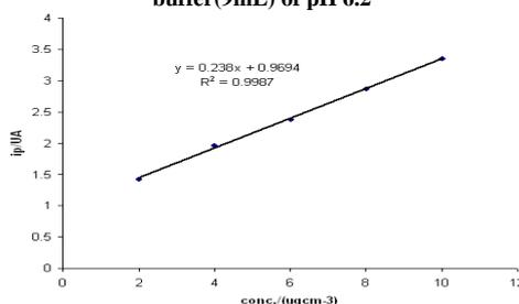
Fig.-9: Plot of  $i_p$  versus concentration from DPCAdS voltammograms in Fig. 8 for AZA in bulk forms
