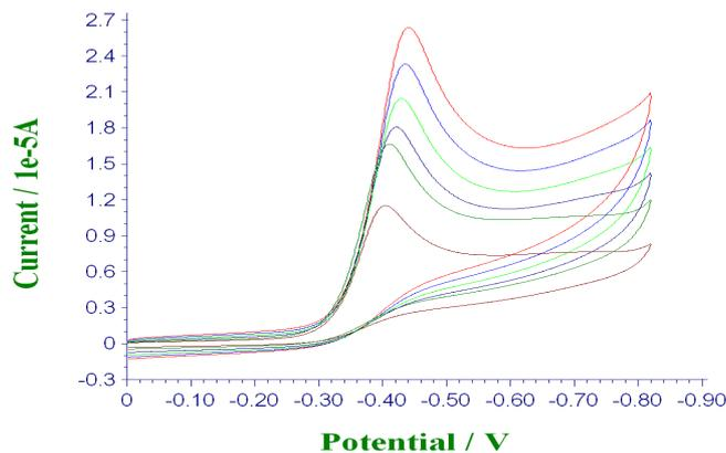
Fig 2: Effect of scan rate on cyclic voltammetric parameters of Azathioprine at pH 6.2 (concentration,  $1 \times 10^{-6}$  M)
