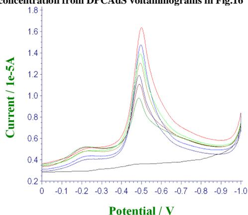
Fig.18: The SWCAdS voltammograms for increased concentrations of azathioprine spiked in serum samples: (1) blank; (2)  $2 \times 10^{-9}$ ; (3)  $3 \times 10^{-9}$ ; (4)  $4 \times 10^{-9}$ ; (5)  $5.5 \times 10^{-9}$ ; (6)  $7.5 \times 10^{-9}$ ; and (7)  $9.5 \times 10^{-9}$ ; and (8)  $1.5 \times 10^{-8}$  mol L<sup>-1</sup>; Eacc.=0.0V, tacc.=15 s, a=50 mV, f=20 Hz,  $\Delta E=10$  mV and BR buffer (9mL)of pH 6.2
