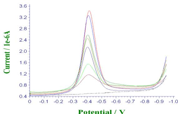
Fig.-12: The DPCAdS voltammograms for increased concentrations of azathioprine spiked in urine samples: (1) blank; (2)  $1 \times 10^{-9}$ ; (3)  $3 \times 10^{-9}$ ; (4)  $5 \times 10^{-9}$ ; (5)  $7 \times 10^{-9}$ ; (6)  $9 \times 10^{-9}$ ; (7)  $1.5 \times 10^{-8}$ ; (8)  $2 \times 10^{-8}$ ;  $\text{mol L}^{-1}$ ; Eacc.=0.0 V, tacc.=15 s, pulse amplitude 50 mV and pulse width 30 ms, and  $\Delta E=10$  mV and BR buffer(9mL) of pH 6.2
