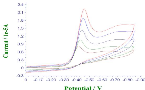
Fig.6: Cyclic voltammograms in pH 6.2 BRB solution on glassy carbon electrode at different concentrations of AZA (1-5):  $1 \times 10^{-6}$ ,  $1.5 \times 10^{-6}$ ,  $2 \times 10^{-6}$ ,  $2.5 \times 10^{-6}$ ,  $3 \times 10^{-6}$  M
