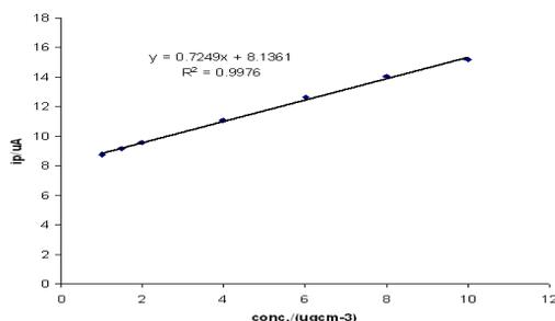
Fig -11: Plot of  $i_p$  versus concentration from SWCAdS voltammograms in Fig.10 for AZA in bulk forms
