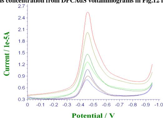
Fig.14: The SW-CAdSV voltammograms for increased concentrations of azathioprine spiked in urine samples: (1) blank; (2)  $1 \times 10^{-7}$ ; (3)  $3 \times 10^{-9}$ ; (4)  $5 \times 10^{-9}$ ; (5)  $7 \times 10^{-9}$ ; (6)  $9 \times 10^{-9}$ ; (7)  $1.5 \times 10^{-8}$ ; and (8)  $2 \times 10^{-8}$  mol L<sup>-1</sup>; Eacc.=0.0 V, tacc.=15 s, a=50 mV, f=20 Hz, ΔE=10 mV and BR buffer (9mL) of pH 6.2
