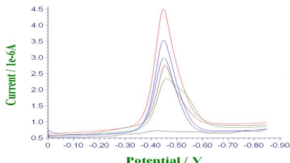
Fig. 8: The DPCAdS voltammograms for increased concentrations of azathioprine in bulk forms: (1) blank; (2)  $2 \times 10^{-9}$ ; (3)  $4 \times 10^{-9}$ ; (4)  $6 \times 10^{-9}$ ; (5)  $8 \times 10^{-9}$ ; and (6)  $1 \times 10^{-8}$ ; mol L<sup>-1</sup>; E<sub>acc.</sub>=0.0 V, t<sub>acc.</sub>=15 s, pulse amplitude 50 mV, pulse width 30 ms, and  $\Delta E=10$  mV and BR buffer(9mL) of pH 6.2
