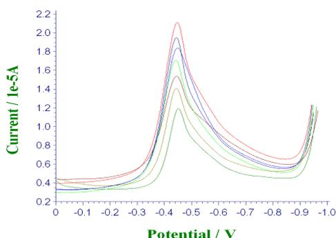
Fig.-10: The SWCAdS voltammograms for increased concentrations of azathioprine in bulk forms: (1) blank; (2)  $1 \times 10^{-9}$ ; (3)  $1.5 \times 10^{-9}$ ; (4)  $2 \times 10^{-9}$ ; (5)  $4 \times 10^{-9}$ ; (6)  $6 \times 10^{-9}$ ; (7)  $8 \times 10^{-9}$ ; and (8)  $1 \times 10^{-8}$ ; mol L<sup>-1</sup>; E<sub>acc.</sub>=0.0 V, t<sub>acc.</sub>=15 s,  $a=50$  mV,  $f=20$  Hz,  $\Delta E=10$  mV and BR buffer (9mL) of pH 6.2
