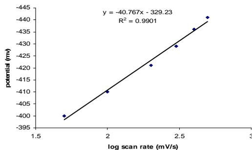
Fig.-3: Plot of  $-E_p$  versus  $\log v$  form voltammograms in Fig. 2 for AZA in concentration at BRB pH-6.2
