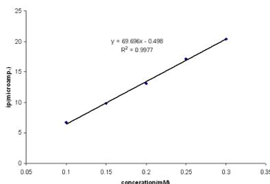
Fig.-7: Plot of  $i_p$  versus concentration from voltammograms in Fig. 6 for AZA at  $100 \text{ mVs}^{-1}$  SR and BRB pH-6.2
