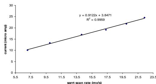
Fig.-4: Plot of  $i_p$  versus  $v^{1/2}$  form voltammograms in Fig. 2 for AZA in  $1 \times 10^{-6}$  M concentration at BRB pH-6.2
