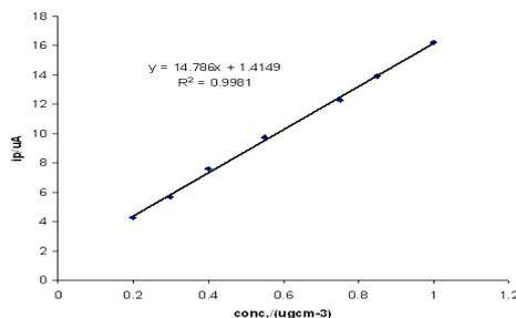
Fig- 19: Plot of  $i_p$  versus concentration from SWCAdSV voltammograms in Fig.18 for AZA in serum sample
