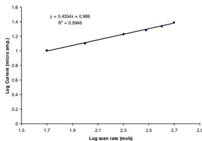
Fig.-5: Plot of  $\log i_p$  versus  $\log v$  form voltammograms in Fig. 2 for AZA in  $1 \times 10^{-6}$  M concentration at BRB pH-6.2
