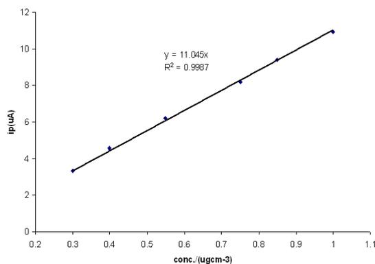
Fig.-17: Plot of  $i_p$  versus concentration from DPCAdS voltammograms in Fig.16 for AZA in serum sample
