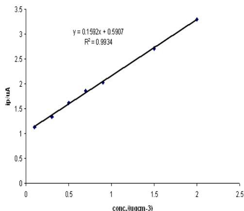
Fig.-13: Plot of  $i_p$  versus concentration from DP-CAdSV voltammograms in Fig.12 for AZA in urine sample
