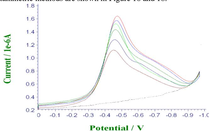
Fig.16: The DPCAdS voltammograms for increased concentrations of azathioprine spiked in serum samples: (1) blank; (2)  $3 \times 10^{-9}$ ; (3)  $4 \times 10^{-9}$ ; (4)  $5.5 \times 10^{-9}$ ; (5)  $7.5 \times 10^{-9}$ ; (6)  $9.5 \times 10^{-9}$ ; and (7)  $1.5 \times 10^{-8}$ ; mol L<sup>-1</sup>; Eacc.=0.0 V, tacc.=15 s, pulse amplitude 50 mV, pulse width 30 ms, and  $\Delta E=10$  mV and BR buffer(9mL) of pH 6.2
