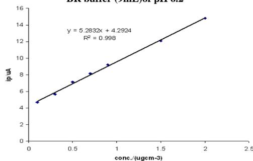
Fig-15: Plot of  $i_p$  versus concentration from SW-CAdSV voltammograms in Fig. 6 for AZA in urine sample
