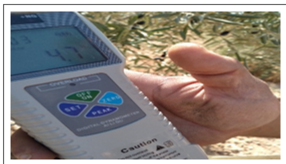
Figure 7: Digital force instruments used for measuring fruit removal force (TPA Plus).
