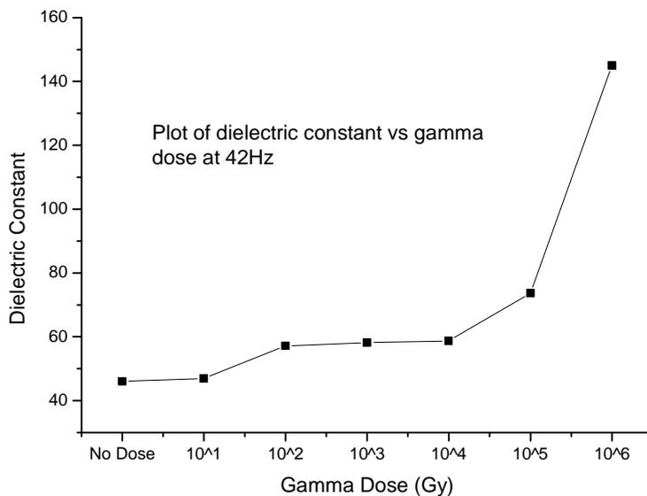
Fig.4 : Plot of dielectric constant at different gamma doses at a frequency of 42 Hz
