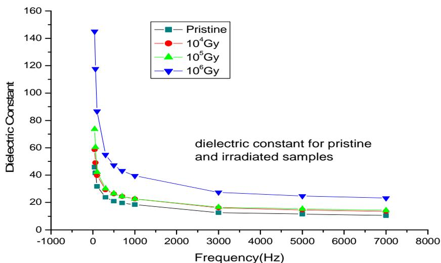
**Fig.2. A comparison of dielectric constant value of pristine and Irradiated sample at different frequencies**
