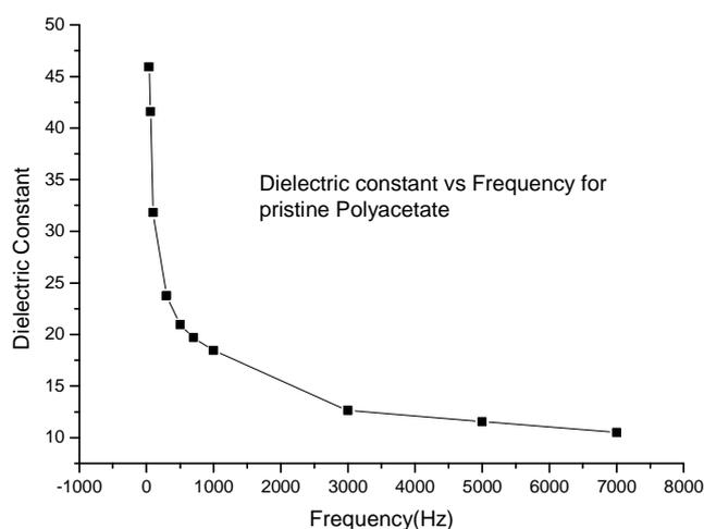
Fig.1. Plot of frequency vs dielectric constant of Polyacetate polymer
