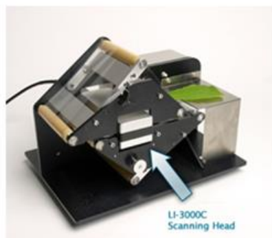
Figure 4: LI-3050C Transparent Belt Conveyor with mounted Li-3000C Leaf Area Meter for measuring leaf area.
