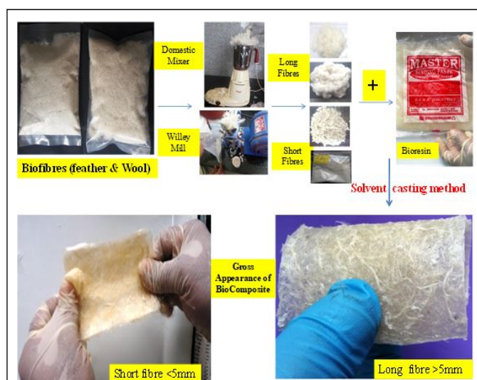
Figure 1: Preparation of biocomposite using keratin biofibres.
