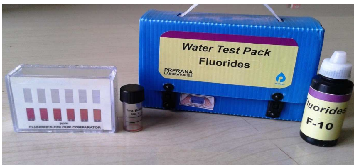
Fig.1 Determination of fluoride in water by using kit
