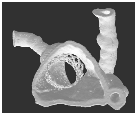
Figure 3: 3D printed model of a human aortic root implanted with a TAVR stent frame showing an area of malapposition responsible for PVL.
