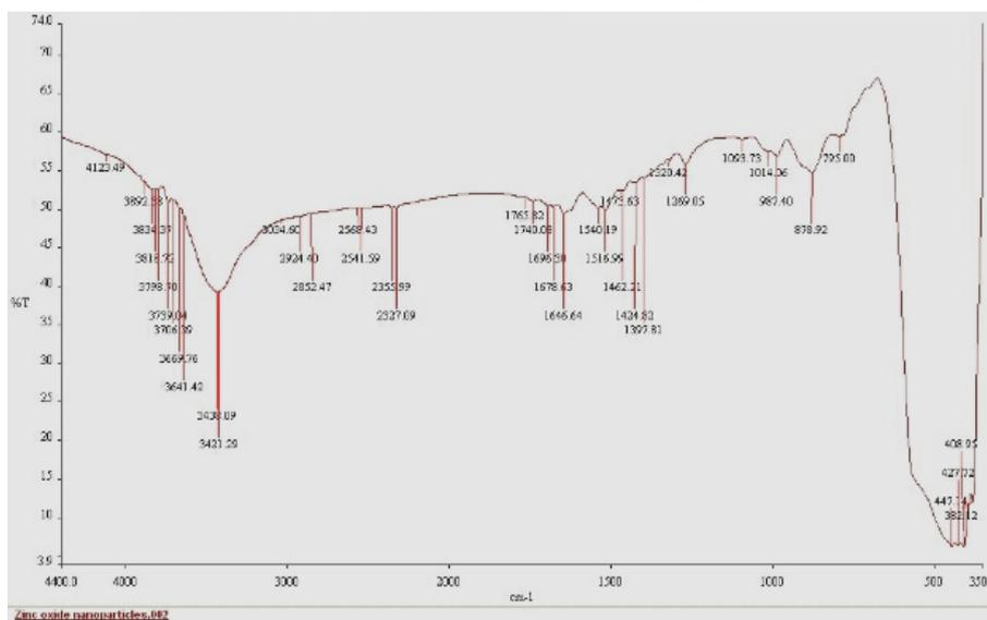
**Figure 3:** FTIR spectrum of ZnONPs acquired in the range of 400-4000 cm<sup>-1</sup>
