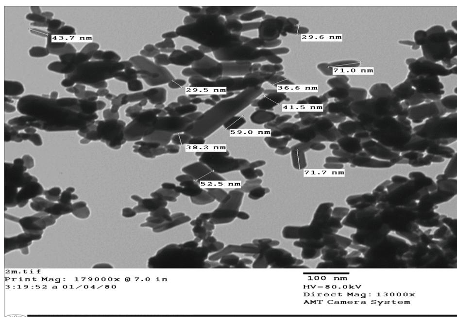
Figure 1: Transmission Electron Microscopy (TEM) of ZnONPs
