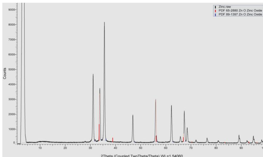
**Figure 2:** XRD pattern of ZnONPs synthesized at calcining temperatures 500°C
