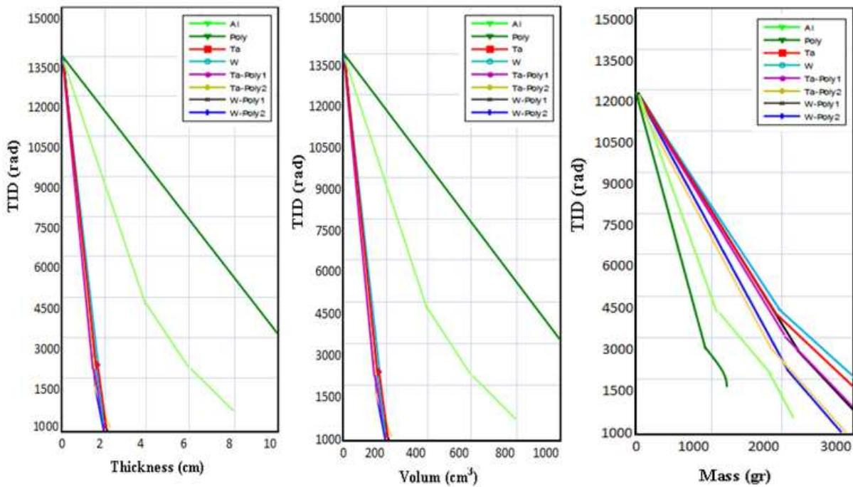
**Figure 6. TID charts in terms of thickness, volume and mass of formation material shielding break the flat shielding**
