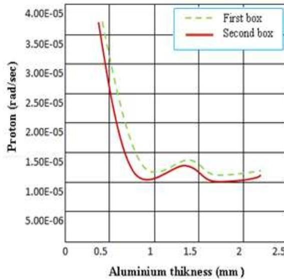
**Figure 3. Aluminum shell thickness according to dose per second**
