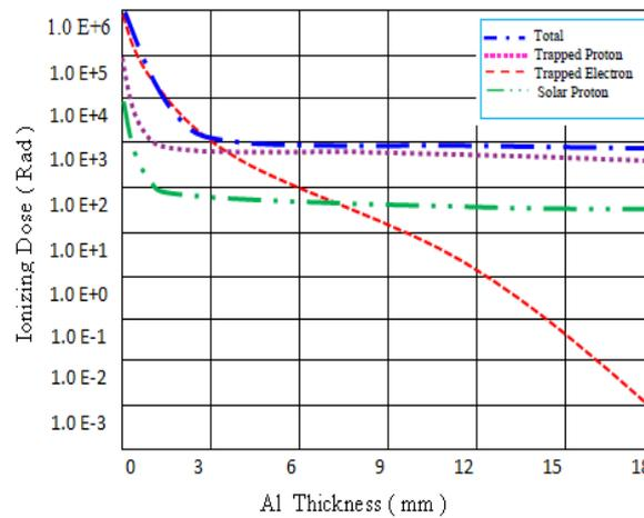
**Figure 2. Doses of ionizing depending on the radiation shield thickness**
