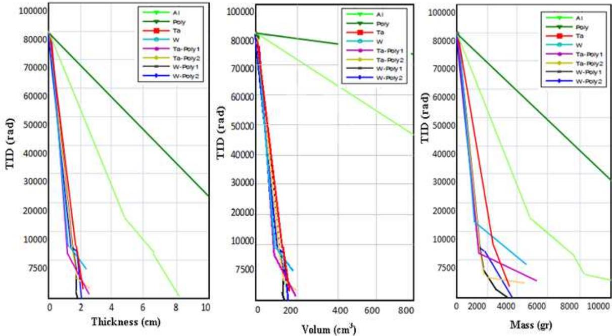
**Figure 5. TID charts in terms of thickness, volume and mass of formation material shielding break the spherical shielding**
