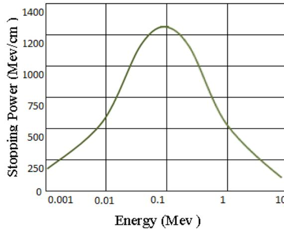
**Figure 1. Stopping power of protons in aluminum**
