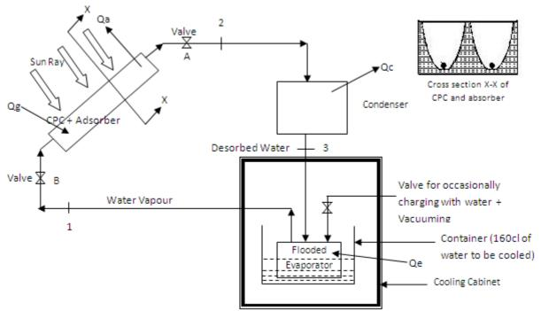
Figure 1; Adsorption Refrigerator Design flow diagrams
