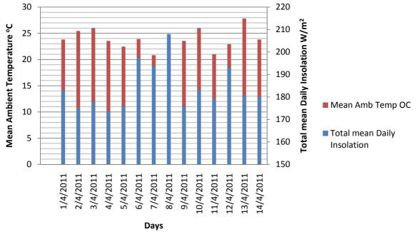
Figure 4: Evolution of Total mean Daily-Hourly Solar Radiation and mean external temperature between (7:00am-17:00pm)for the experiment
