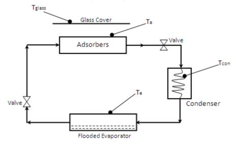
Figure 2: Flow diagram and Instrumentation
