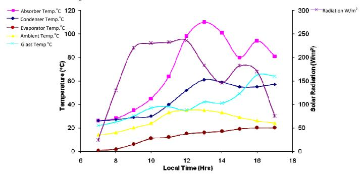
Figure 3: Day 1(1st April 2011) Hourly variation of Solar Radiation and system temperature in a day
