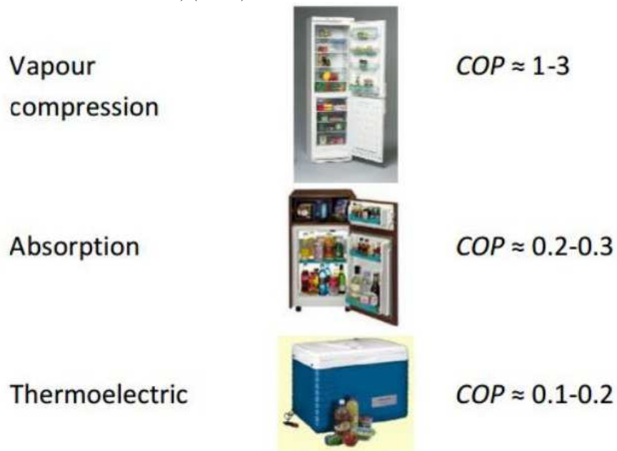
Figure 1: Different cooling principles and their typical efficiency. COP is a quality number defined as the ratio between the useful cooling energy and the supplied work
