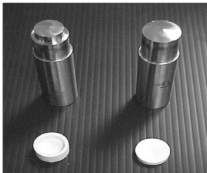
Figure 4. Photo of the tooling used to demonstrate proof-of-concept, a cup, and a finished dosage form
