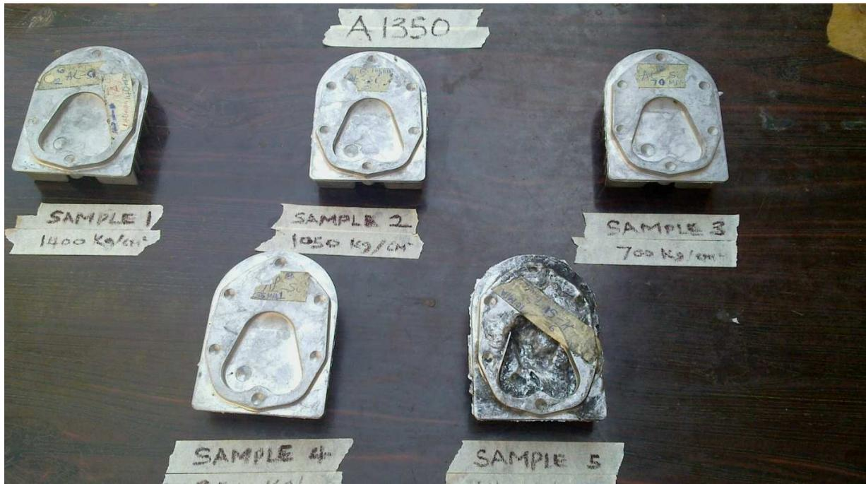
Figure 1: Samples of A1350 after casting
