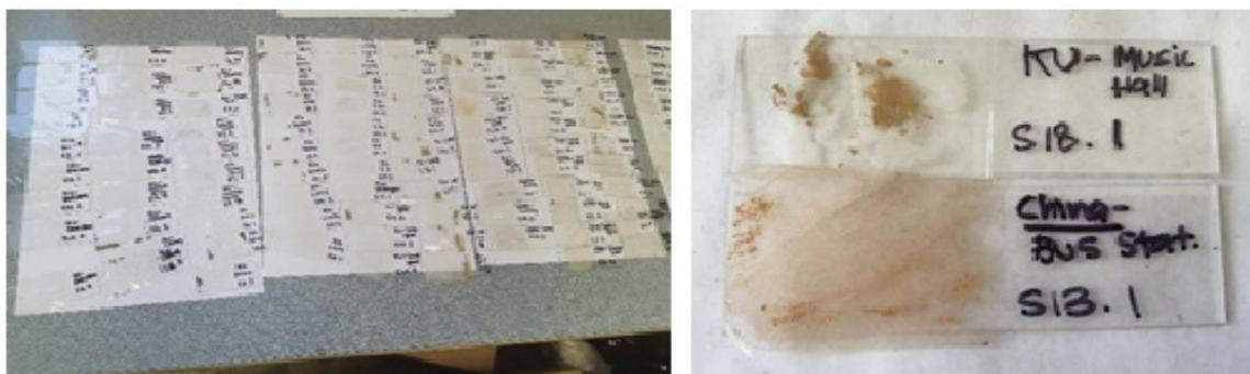
**Figure 2:** Slides of tree leaf samples prepared for microscopic analysis.
