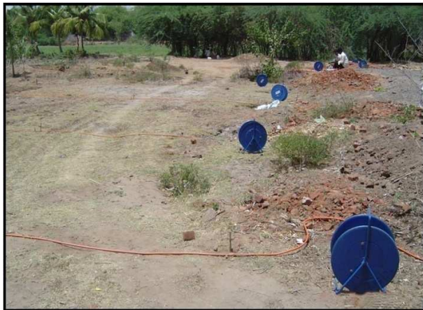
Figure 4.4 Multi-electrode winch set-up
